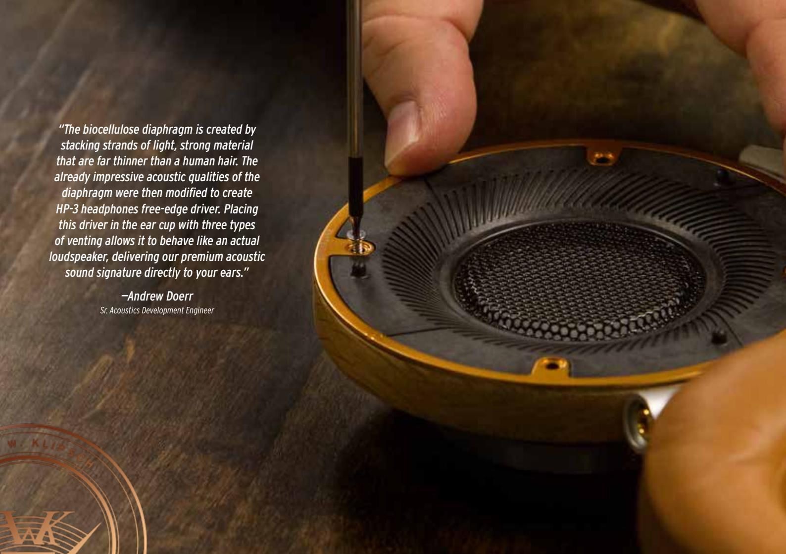
*"The biocellulose diaphragm is created by stacking strands of light, strong material that are far thinner than a human hair. The already impressive acoustic qualities of the diaphragm were then modified to create HP-3 headphones free-edge driver. Placing this driver in the ear cup with three types of venting allows it to behave like an actual loudspeaker, delivering our premium acoustic sound signature directly to your ears."*
