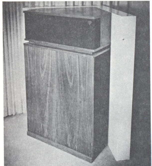
FIG. 2. Complete, free standing false corner as described above.
