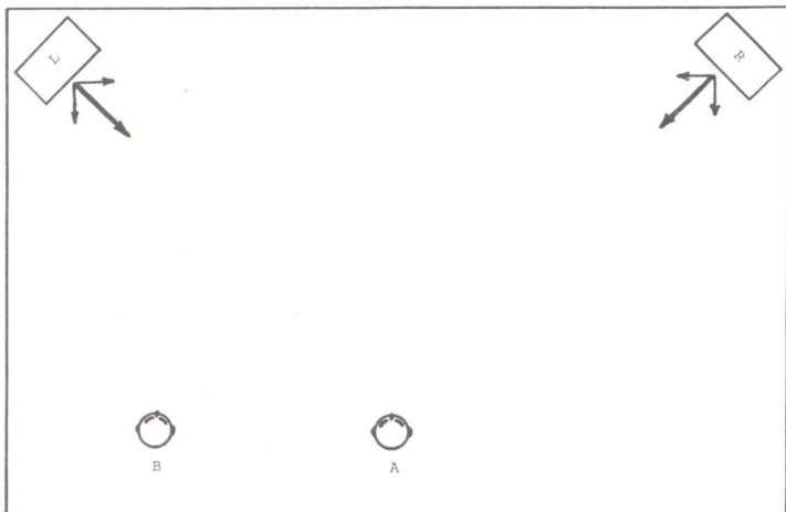
Fig. 3 Toe-in of Loudspeakers Resulting in Improved Retention of the "Stereo Effect" over a wider Listening Area.
