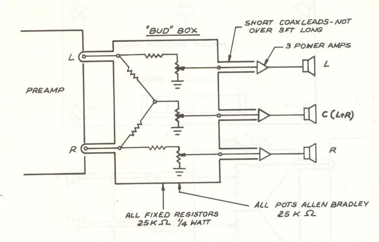
MATRIX CIRCUIT FOR 2-3 STEREO : TWO CHANNELS TO
